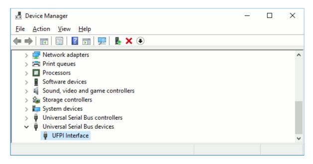
On Windows XP/Vista/7 without installed WCID support the simplest way to install driver in one click it's a Zadig software. Download Zadig, connect UFPI interface and press "Install WCID Driver". Screen shot below illustrates driver install using Zadig.
